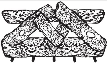
**Important:** Adequate ventilation is absolutely necessary. Adequate spacing between the logs is **NECESSARY and MUST be maintained**. Some carbon build up (sooting) may occur where flames strike the logs. If carbon build up (sooting) continues, rearrange top logs to allow more opening(s) for flame(s) before sooting becomes worse. **If any sooting occurs outside of the firebox (i.e. on the walls), turn off unit immediately and contact a qualified professional service technician.**
